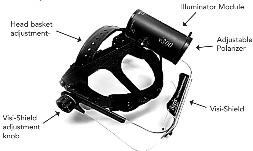
Figure: 2 v300H Component Parts
